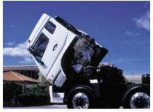
Electric hydraulic tilt mechanism for easy engine maintenance.
