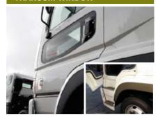
Improves LHS driver visibility for easier, safer parking and manoeuvring. (Except FP430G8). 3 step entry and doors and step lights for easy access.
