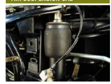
Cab suspended on 4 point air suspension with 2 auto levelling valves and pan hard rods for driver comfort. (Except FV370K8 & FP430G8)
